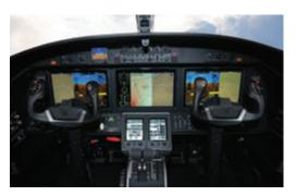
It maximizes aircraft performance with precise lateral and vertical navigation guidance for all phases of flight, as well as pinpoints fuel calculations thanks to the autothrottles.
